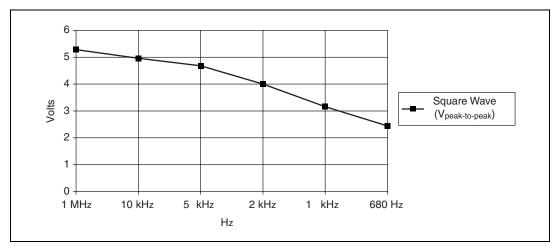
Figure 3. Typical Maximum Voltages versus Load Impedances
